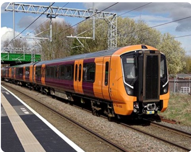
Source: 3-Car Class 730 Electric Multiple Unit from the Corelink fleet
